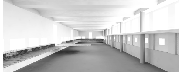
Figure 4: A model of the computer room in the Queen's Building at De Montfort University used to predict DFs and assess the effect of light shelves
